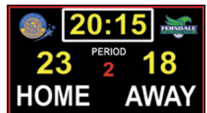
2560mm x 1440mm (4 x 3 cabinets) P5 Resolution: 512 x 288 pixels
