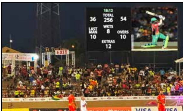
Combining Scores and Video on this large Cricket Scoreboard - 13 metres by 6 metres
