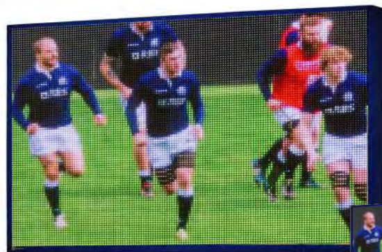
20mm pitch 150 x 100 resolution 3 x 2 metres Above viewed at 6 metres - Too Close!
